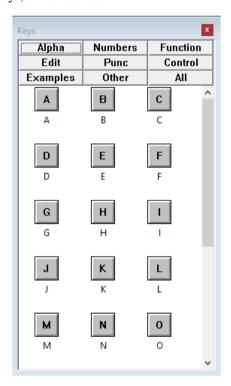
**Technical Note:** The Keys window is managed by the KEYS.INI file in the BIN folder - the actual Keys shown, and the default labels and actions are contained within this file, and is relatively easy to modify for the technically minded - syntax notes and details are listed as comments in
