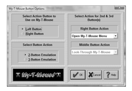
**Important:** The term Mouse is used generically for any pointing device that moves the cursor (mouse pointer) within Windows. For Pen and Touchscreen drivers, often only 1 button is available (Left Button): In all cases, the Left Button should be selected as the Action button.
