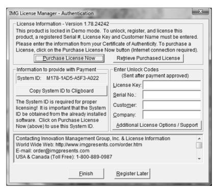
The License Key and Serial No. entries are a matched pair, and will work together to unlock the software. The Customer entry is required (i.e. some text must be entered in the Customer text area), but is not part of the license unlock process. The Company text area is optional, and will be shown as the Source when the product is licensed.
