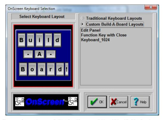
There are a few sample, custom Build-A-Board Layouts available. Additional Build-A-Board layouts can be created, and when placed in the Installation Folder will be added to this list. When selected, the KEYBOARD.KBF in the users configuration folder is replaced with the selected layout. When OnScreen is run, the layout is recognized, and the Build-A-Board compatible run-time (MYTSOFT2.EXE) is used to operate with the version 2.x keyboard layouts.
