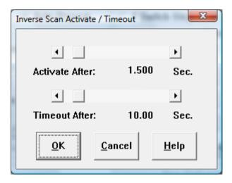
The Inverse Scan uses the Mouse or Joystick button as a stop/go control. When the selected device button is down, scanning will continue, and when up, scanning will stop. The click is automatic based on settings in the Inverse Scan Activate / Timeout dialog. After a stop for the activation time, the next step in the CrossScanning process will occur (see Auto Scan). If there is no go signal (button down) during the Timeout time, the scan will be stopped.
