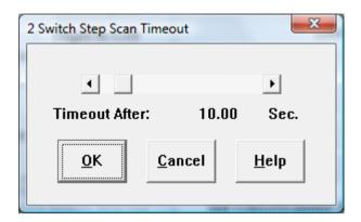
The 2 Switch Step Scan uses the Mouse buttons as a stop/go control and a click. When the Left Button is selected, the Right mouse button will be a stop / go control for the CrossScanning scan, and the Left mouse button will be the click to advance in the CrossScanning process. If Right Button is selected, the Left mouse button will be a stop/go control for the CrossScanning scan, and the Right mouse button will be the click to advance in the CrossScanning process.
