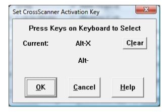
The Activation key is used to toggle CrossScanner from an active mode (awake), to an inactive mode (sleeping) while CrossScanner is running within Windows. Within Setup, you may select the Activation Key (or combination of keys) used to Activate/De-Activate CrossScanner. You may use keys F1 through F12, 0 through 9, and A through Z, by themselves, or in any combination with Ctrl, Shift, and/or Alt. Make sure CrossScanner is not running when you select the Activation Key.
