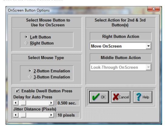
**Important:** The term Mouse is used generically for any pointing device that moves the cursor (mouse pointer) within Windows. For Pen and Touchscreen drivers, often only 1 button is available (Left Button): In all cases, the Left Button should be selected as the Action button.
