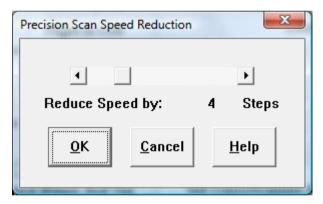
The Precision Scan option is similar to the Auto Scan option, except it adds in extra clicks to slow down the scanning during both the LineScan and FingerScan. When selected, you have the option of selecting how much to Reduce the Speed (from the current selected speed for the type of Scan (LineScan/FingerScan) in Precision Scan Speed Reduction). For each scan, the sequence goes as follows:
