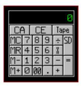
The calculator is a standard four function calculator. To operate simply press the desired number, press an operation key, press the next number, and press an operation key or the total (=) key. You may then send the displayed number to the active window by pressing the SD (Send) button. While there is a number stored in memory, the calculator's display window frame will change color to indicate that memory has a value stored.
