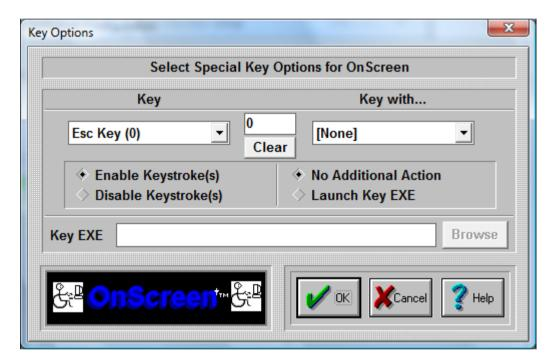
Key Options offers customization capabilities for keys on the main Alpha Keyboard Panel and the Edit panel. Keys may be disabled, assigned to other functions, and can be re-mapped using the Launch Key EXE in conjunction with the Developer's Kit (e.g. the Esc key could be re-mapped to send Alt-F4).
