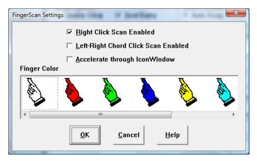
Enabling Right Click Scan Enabled allows FingerScan to 'bounce' off of the right edge of the CrossScanning area and 'become' a right click. This feature is enabled by default. The Left-Right Chord Click Enabled allows a third scan of the screen (After the right-to-left Right Click Scan). This allows the action of simultaneous Left & Right button clicks together (so named from the musical analogy of a Chord). Certain applications use this, and it has been included for completeness.
