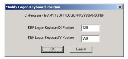
If you do not have Build-A-Board, and wish to change the opening position of the Small/Medium/Large Build-A-Board layouts, there is a basic utility called KBFLOGON.EXE in the LOGON folder. You can access this by clicking on **Update Opening Position** (**Build-A-Board Layouts**). By running this utility, you can change the opening X / Y position of the current selected Build-A-Board layout to match your screen orientation & resolution.
