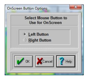
**Important:** The term Mouse is used generically for any pointing device that moves the cursor (mouse pointer) within Windows. For Pen and Touchscreen drivers, often only 1 button is available (Left Button): In all cases, the Left Button should be selected as the Action button.
